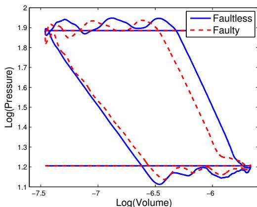
Figure 1. Logarithmic pV diagrams of measurements from faultless and faulty valves
